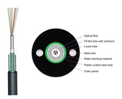
Suitable for long-distance communication and inter-office communication. The two parallel steel wires not only resist tension but also resist lateral pressure, and the optical cable has good mechanical properties. The optical cable has small outer diameter and light weight, which is suitable for construction.
